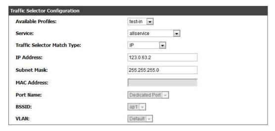
You can see the inbound IP address has to setup speedtest source IP address. (123.0.63.2)
